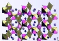
Structure cristalline de \text{Na}_3\text{Fe}_3(\text{PO}_4)_4
